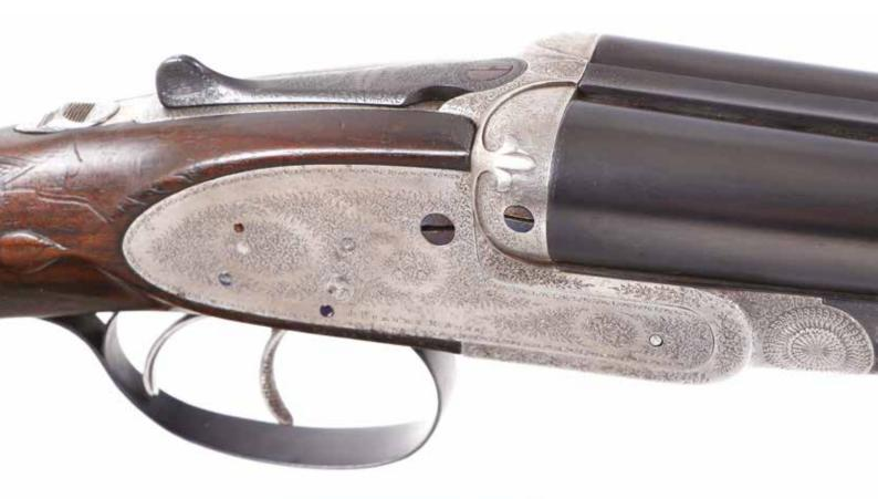
(S2) 12 bore assisted-opening sidelock-ejector by J. Purdey & Sons c.1882, 29½ ins chopperlump barrels, choked at ic & ¼, the top rib inscribed J. Purdey & Sons Audley House South Audley Street London Made Of Sir Joseph Whitworth's Fluid Pressed Steel, 2½ ins chambers, fine border scroll and bouquet engraved action and locks inscribed J. Purdey & Sons, well-figured 14¼ ins straight hand stock, weight 6lbs 11oz, no. 11264 Est £2500 - £3500
